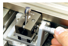
Device for the fine tuning of the slide position, with micrometric head, 0.5 mm/rev pitch, \pm 6.5 mm range
