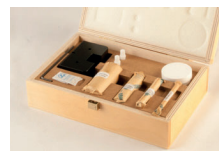
Set of 4 calibration pins for XLS40 micrometer, with supporting V block.
