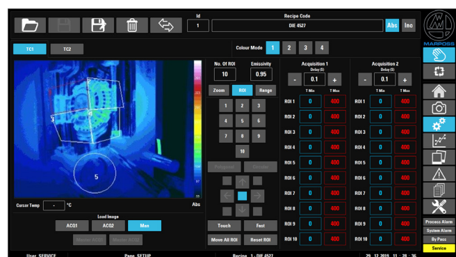
Thermographic image with temperature values for each ROI and recipe setup parameters
