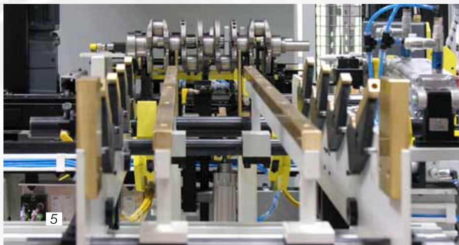
3 - ND check on camshaft 4 - Self-mastering device 5 - Rejected parts chute
