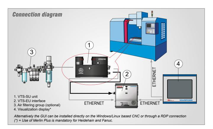
The VTS GUI is the graphic interface software of the system, that in ECHO mode displays the image and the result of the measurement that the machine cycle has generated. It can be installed on the CNC (Windows/Linux based), and on the PC and communicated with the VTS through an Ethernet connection. The images can be viewed on the CNC screen or on an external computer, such as Merlin Plus.
