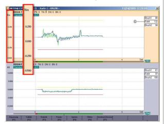
DDU-rotor and DDU-stator constitute the sensor system for contact-free monitoring of rotating and rigid tools. In combination with the relevant measuring transducers, the system is employed with all ARTIS tool and process monitoring systems. The figure shows an example for use in the CTM system.
