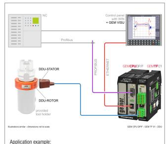
GEMTF01 Torque and Axial Force Measuring transducer with a **DDU-Rotor**, a **DDU-Stator** and the GENIOR MODULAR Tool and Process Monitoring System.
