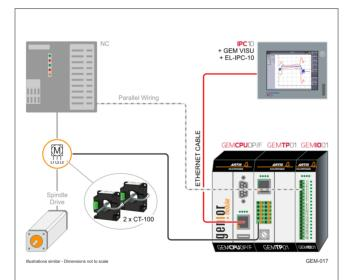
Application example: Parallel wiring between the GENIOR MODULAR Tool and Process Monitoring System and the machine control using a GEMIO01 Input-/Output-Converter, e.g. for true power monitoring (with 2 CT-100 Hall sensors and a GEMTP01 measuring transducer module).
