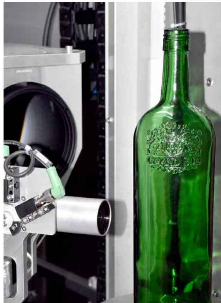
wall thickness measuring station
