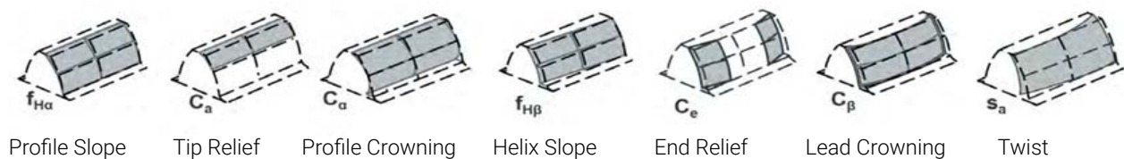
Figure 2 - Possible modifications to the shape of tooth flanks of involute gears [3]
