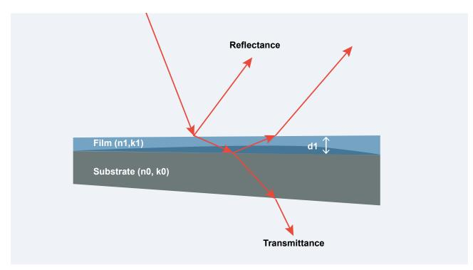
This interference results in constructive and destructive patterns, which appear as oscillations in the wavelength-dependent reflectance spectrum.
