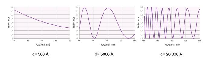
Two primary data analysis methods are employed to extract the layer thickness.
