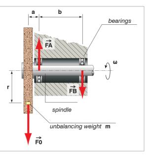
If the grinding wheel operates constantly while imbalanced, vibrations are continuously transmitted to the machine's mechanical parts, particularly the spindle and the bearings, and with time may damage the machine tool and cause a deterioration in its mechanical integrity.
