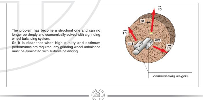
All grinding wheels are normally balanced manually by the operator positioning compensating weights in the appropriate positions on the grinding wheel flange, although this operation requires skilled personnel and lengthy periods of time if it is to be carried out in a correct and effective manner.
