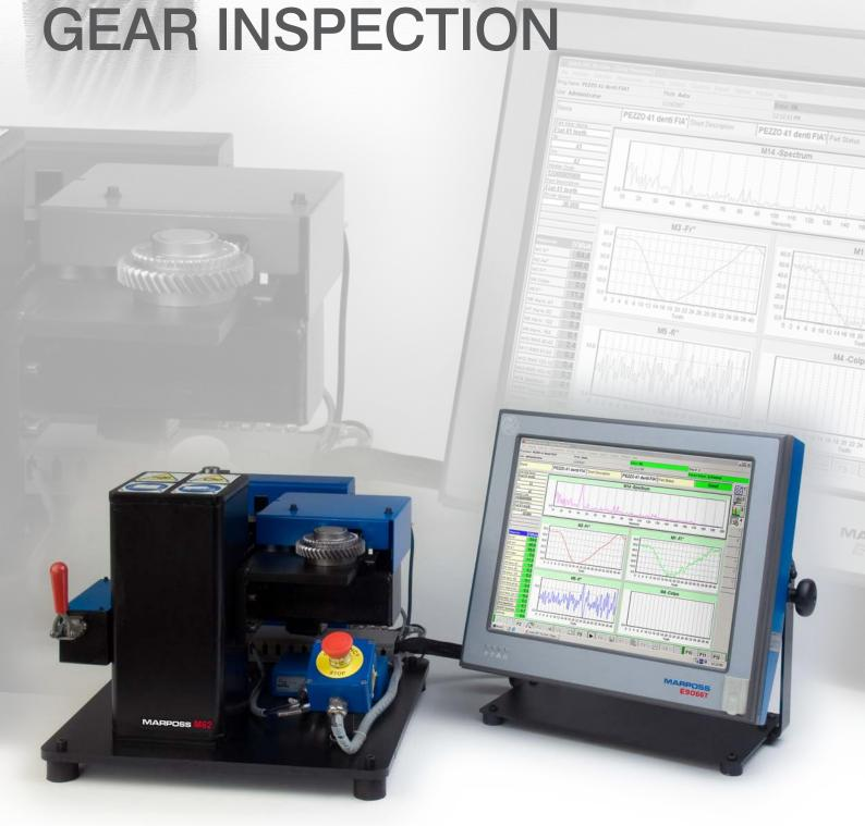
The M62 DF Micro is an accurate gauging instrument conceived for the double flank inspection of spur and helical gears with pitch diameters ranging from 20 to 120 mm. The system is designed to be simple and easy to use for the operator in the shop floor environment. The typical parameters can be quickly evaluated in numerical values and graphic visualization on the E9066T Thin Panel Industrial Computer.
