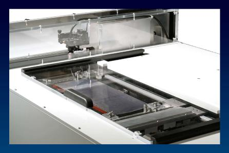
Specifically designed for Li-Ion Battery Analysis, Lab Sense combines different sensors able to precisely determine weight, thickness, and density. This system was born in response to the needs of our customers, who seek a complete quality control system. As ultrasonic technology pioneers for basis weight and confocal technology within Marposs Group, our solution is able to completely track the geometry of your battery foils providing a robust and accurate quality control system.
