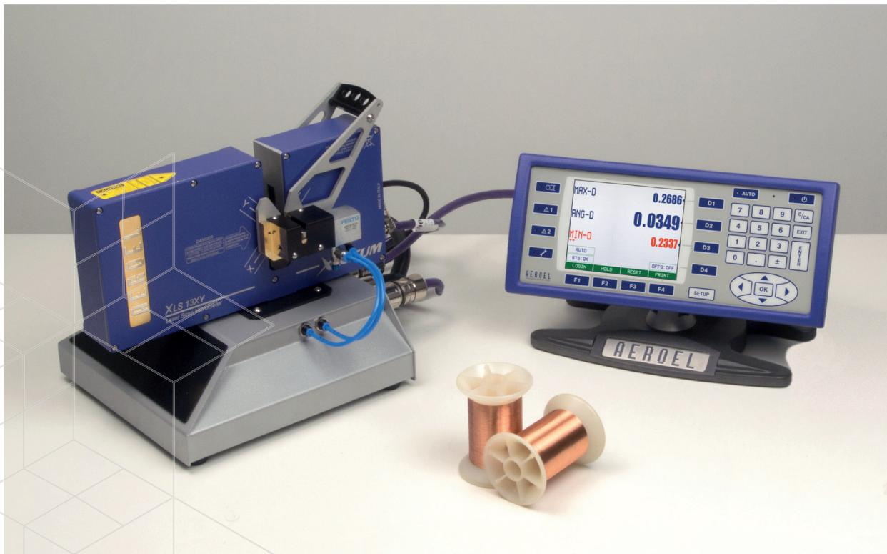
**WIRELAB.XY** is a high performance table-top laser micrometer designed to be used off-line to check drawn or extruded products, when diameter and ovalization must be accurately measured. It is the ideal instrument to measure wire samples, optical fibers and magnet wire or to check the die diameter by measuring the drawn wire.
