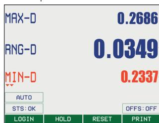
geometry of the section, taking several readings, all along the 360° of the sample circumference. The maximum and minimum diameters are retained, as well as the Max-Min value, which is the true ovality of the sample.
