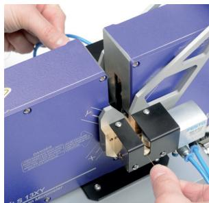
Using a special fixture to manually rotate the part, the diameter can be measured over  $360^\circ$  of the circumference to precisely measure the maximum MAX-D, the minimum MIN-D and ovality which is really MAX-D - MIN-D.
