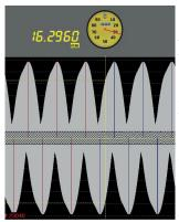
Using a special guided procedure, the operator seeks the starting point, moves the part to the measurement position and starts the measuring cycle: the part is rotated by a special motor driven device using a rubber wheel laying on the part. This keeps it pushed against the V blocks and assures a "zero runout" rotation, that is a rotation around a perfectly fixed axis.
