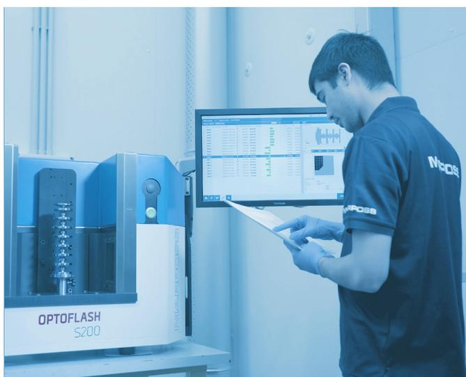
The periodic calibration is executed through a dedicated software tool and specific masters that allow a fine tuning of the product mappings, directly on site.
