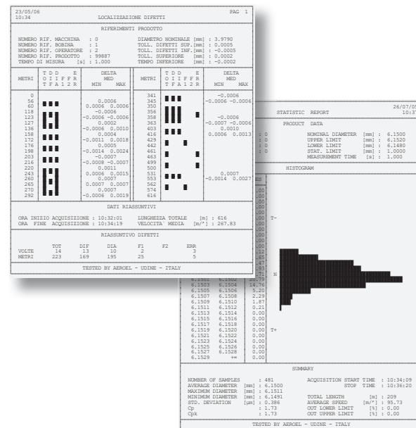
(\*) Only flaws which turn into a diameter change all along the product circumference, like "olives" or "neck-down", can be surely detected. The minimum detectable flaw length is given by the max line speed divided by the gauge scan frequency.
