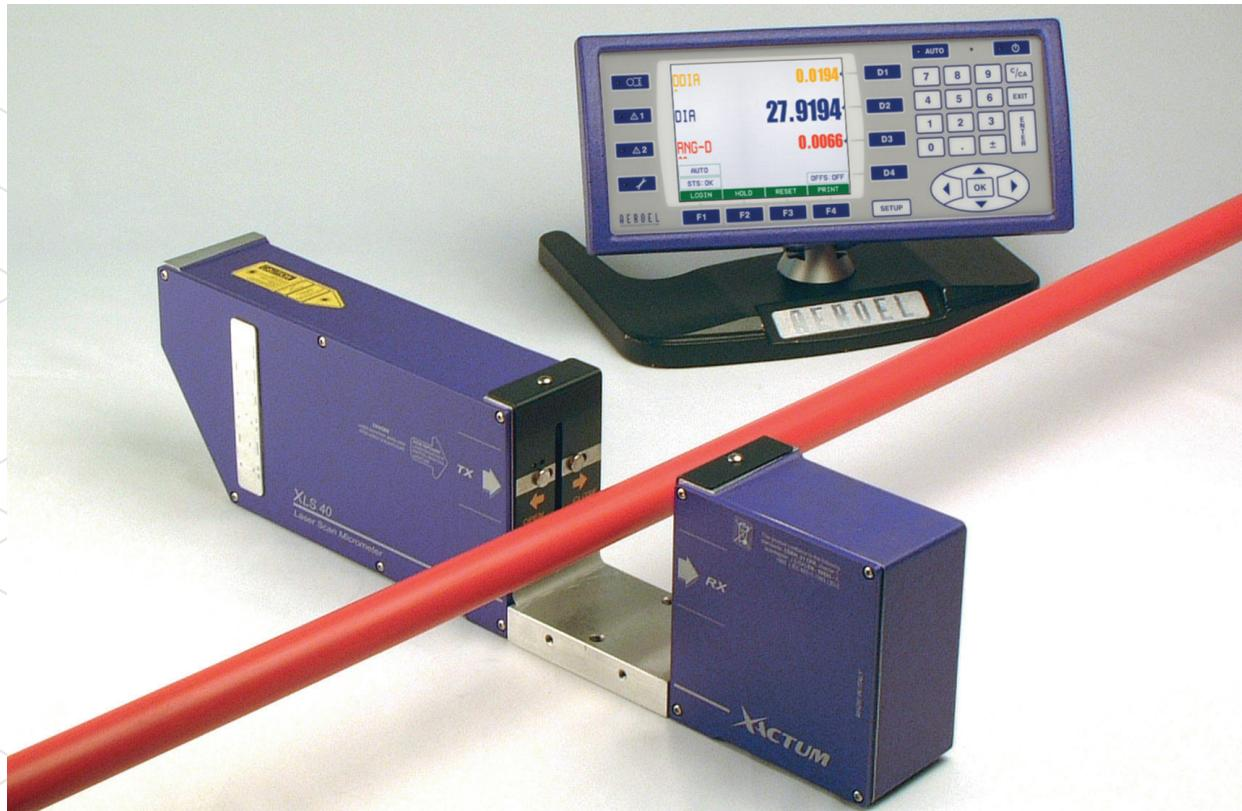
**Extruline.X is a laser system designed to control the external diameter of extruded products such as electrical wires, plastic tubes and similar products.**
