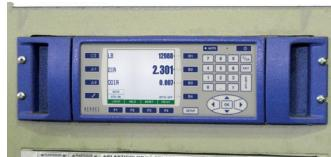
Panel, the operator uses function keys and pop-up menus to select the various functions or to enter the numerical values requested by the program.
