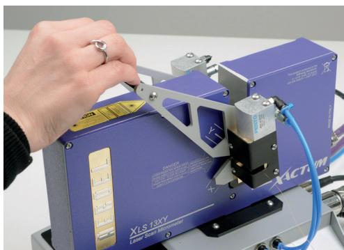
The measured values are displayed on a highly visible backlit LCD display. They are compared with the tolerance limits to check the dimensional conformity of the part. The collection of measurements along the circumference allow also to draw a polar plot of the circular sections.
