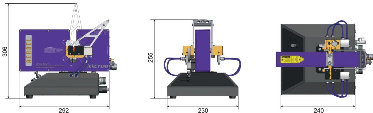
All dimensions are in mm. Dimensions without cables and connectors.
