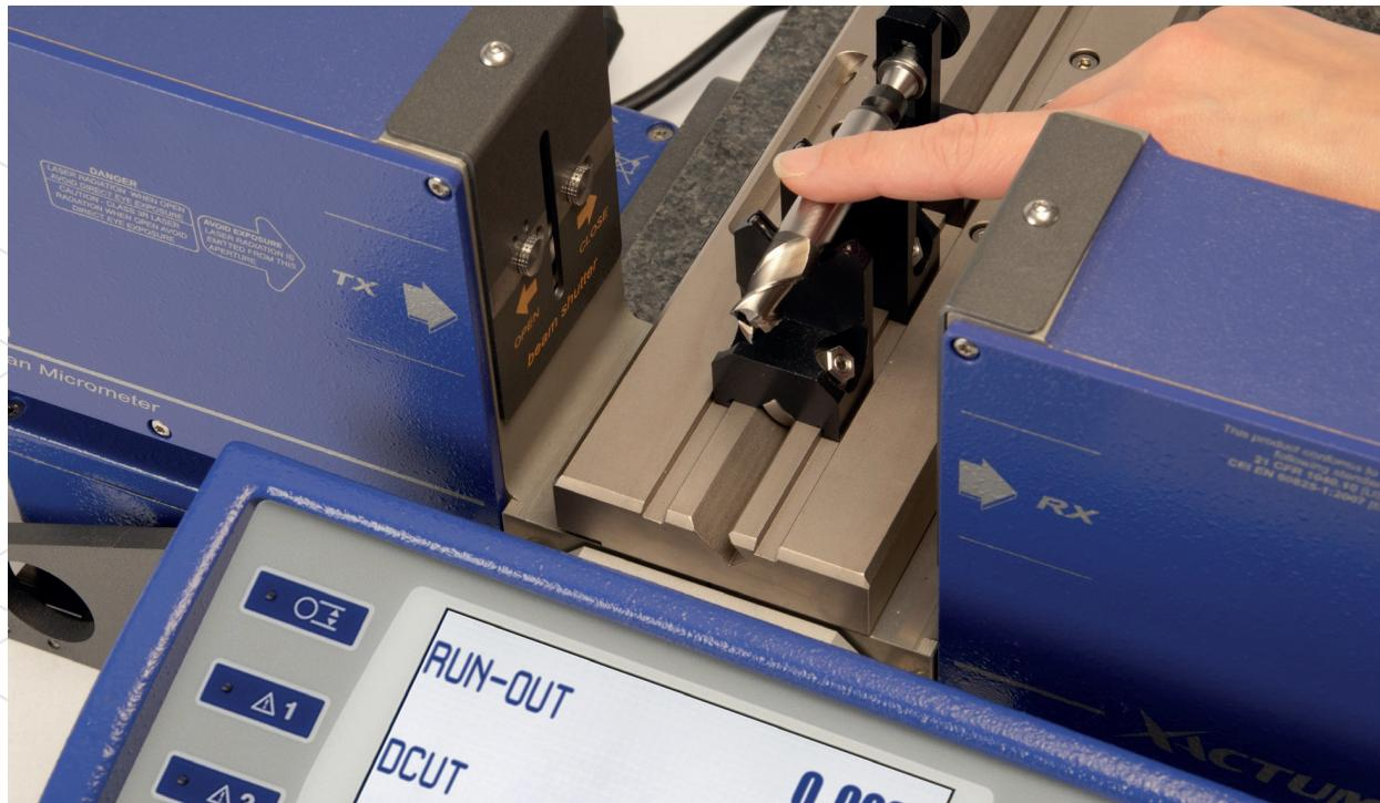
MECLAB.T40 is a high precision laser instrument for quick and simple diameter measurements of hard metal blanks and full carbide cutting tools, odd or even edges. It's ideal for the off-line checking of
