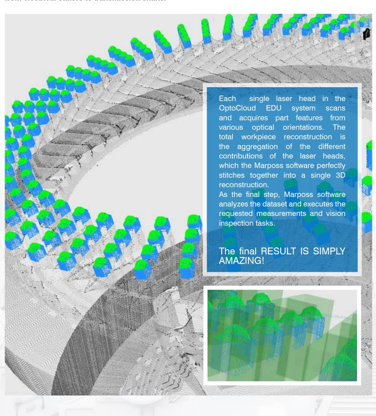
Large, complex surfaces are acquired at very high resolution within seconds. Using the extensive dataset of surface points, the OptoCloud can execute a super-precise surface digitalization, which is then processed by the Marposs measurement and inspection software engine.
