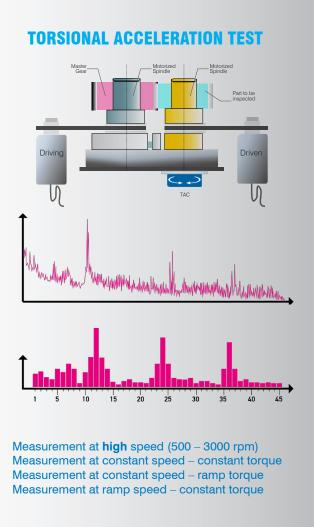
The output parameter is the **angular acceleration** (rad/s<sup>2</sup>) evaluated instantaneously and in the long run.
