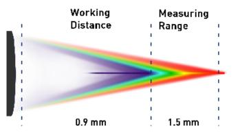
Working with any STIL optoelectronic controller, the ENDO series allows precise measurements with a sub-micron resolution.
