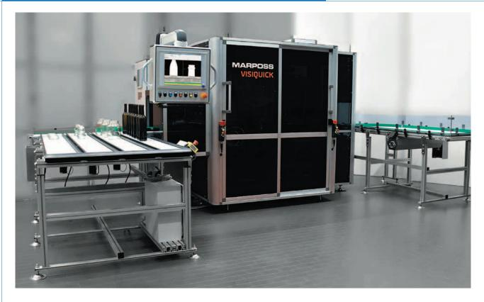
technology, on round, square and rectangular containers and labelling area profile, a solution patented by Marposs that allows to detect and measure, sinks and bulges on the areas of the container where the label has to be applied. Sinks and bulges can be responsible for wrinkles or bubbles when the label is applied.
