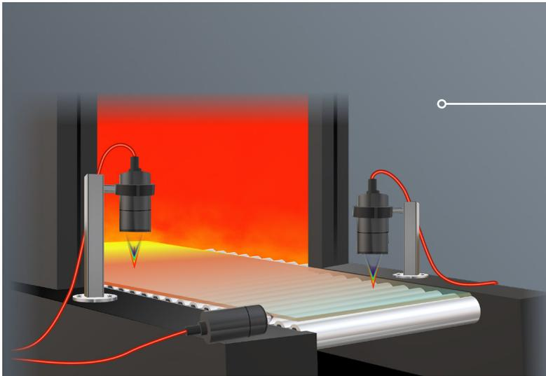
**Hot glass thickness & shape measurement**
