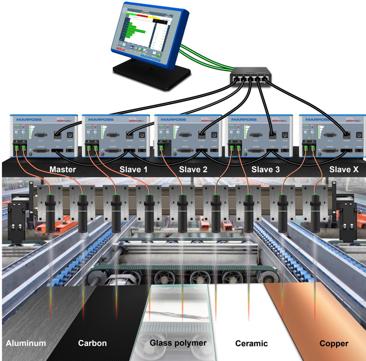
ZENITH™ controllers with 1 or 2 measurement channels, can be synchronised at up to their maximum frequency (in occurrence 20 kHz) within a Master-Slave configuration. Measurement synchronisation of all controllers is then done via the “Trigger In” & “Trigger out” pinned on Interface connector. The controller working at the slowest frequency defines the tempo.
