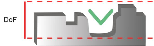
Depth of Focus, also called Depth of Field or DoF, is defined as the distance (on Z-axis) where all points are well resolved so that image elements are distinguished, understandable & usable.
