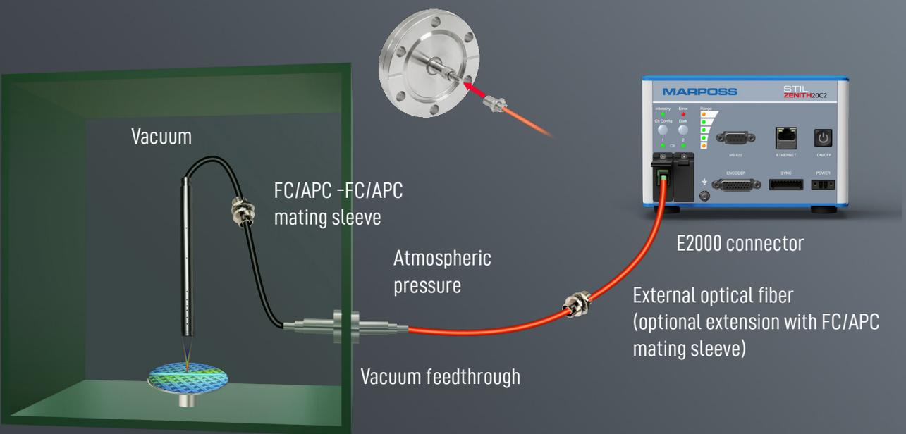
Optical pen, vacuum compatible. Optical fiber, FC/APC vacuum compatible
