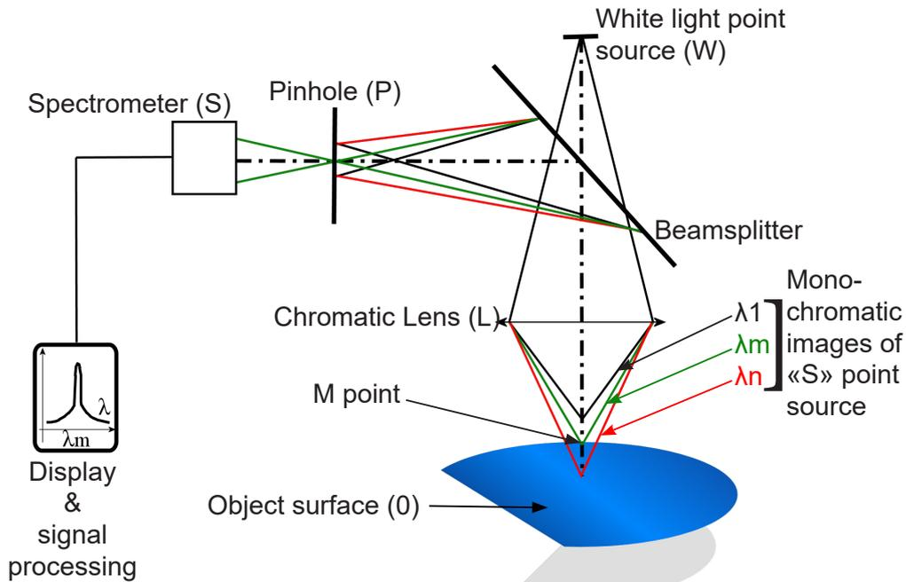
A pinhole of incident white light is transformed, through a chromatic lens, into a continuum of monochromatic images along the Z-axis, thus providing a «color coding» along the optical axis. When an object is present in this «colored» field, a single wavelength is perfectly focused on its surface and then reflected in the optical system.
