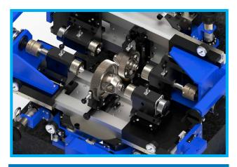
Marposs Single Flank system for use in the Laboratory to test prototyping parts with the purpose of feedbacking the gear design process. The system has the capability of testing either part vs master gear or part vs the conjugate gear as in the real transmission (reducer). The operator even has the possibility to adjust both center distance and angle of inclination of the axis in order to obtain the configuration leading to the minimum noise contribution.
