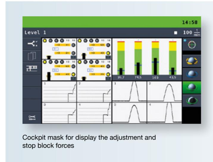
Cockpit mask for display the adjustment and stop block forces
