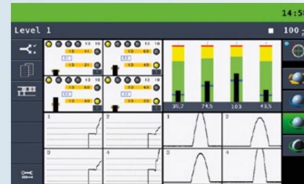
Cockpit mask for display the adjustment and stop block forces
