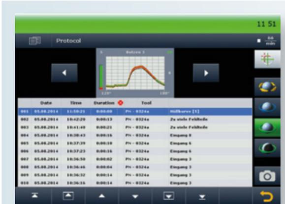
The device protocol records failure curves together with all process data.
