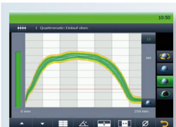
X5 displays and monitors the rolling forces for easier analysis over the tool length (mm).
