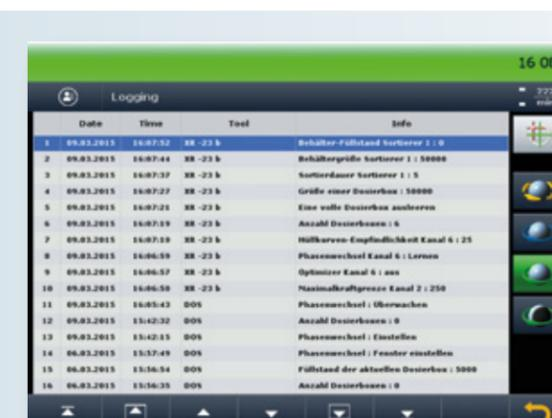
This protocol stores the last 250 operator inputs with the date, time and the used tool number.
