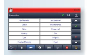
From configurable actions the relevant stop codes can be displayed and selected by the operator. In case of missing user input, the machine can be locked.
