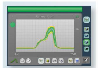
The "Optimizer plus" automatically determines the optimum sensitivity (envelope width) for the entire envelope curve.
