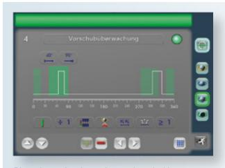
Binary input signals can be monitored with up to three monitoring windows to ensure the earliest possible fault detection.
