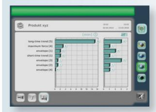
The failure distribution shows machine downtimes and the frequency of process failures for a quick and easy failure analyze.
