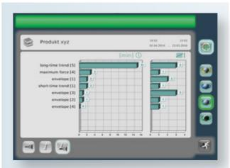
The failure distribution shows machine downtimes and the frequency of process failures for a quick and easy failure analyze.
