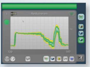
The "Optimizer plus" automatically determines the optimum sensitivity (envelope width) for the entire envelope curve.
