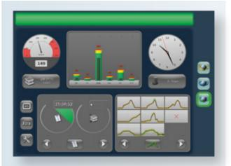
X7 Cockpit: Switchable mask design with flexible arrangement of the monitoring channels (according to the machine configuration).
