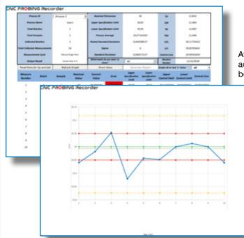
At the end of production, the data collected can be saved automatically and exported in Q-DAS format so it can be processed in the future using software for statistical
