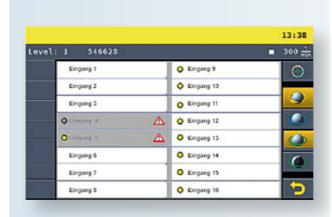
Up to 16 binary feed, ejection, and coil end sensors are visualized and monitored in an overview mask.
