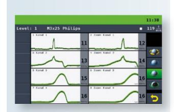
The X1 performs an automatic calculation of the monitoring windows for new products.
