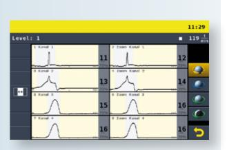
The multi-channel mask shows all process signals including envelope curves, choosen settings and process stabilities.
