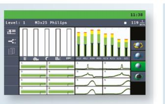
The cockpit mask provides all relevant information at-a-glance: counter readings, maximum forces, envelope curves and trend limits.
