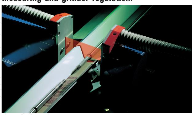
The Grindline.X Laser System has been specially designed for on-line gauging of the outside diameter of products manufactured by through-feed centreless grinding machines, like pins, shock absorbers rods, steering racks or any other part having one ground diameter only to be checked.
