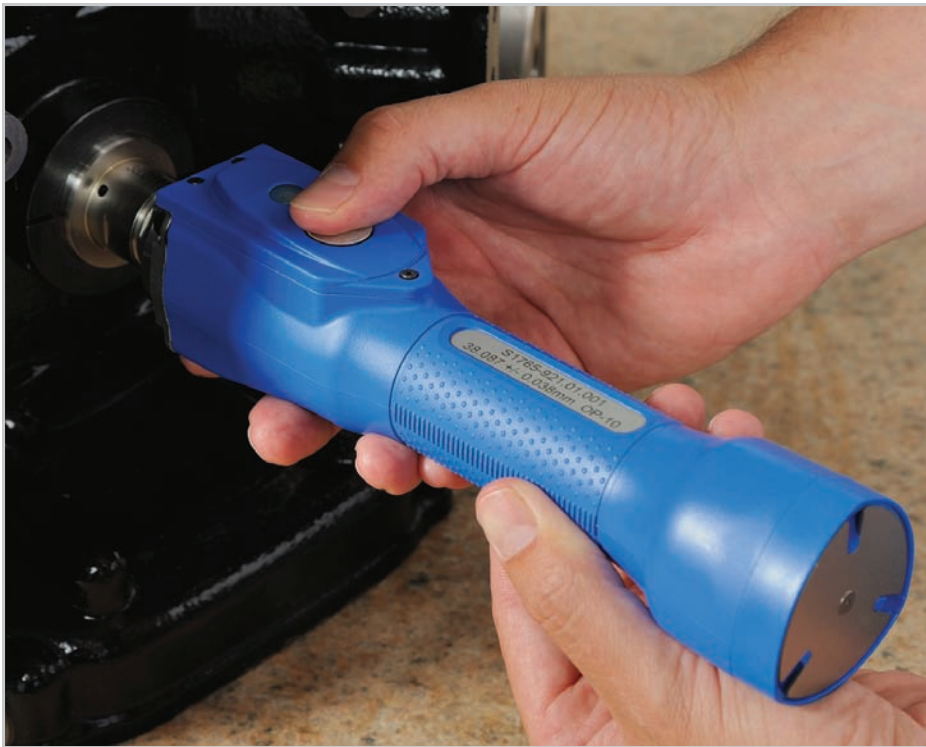
Wave bore gages embedded with Bluetooth® wireless technology may lower overall inspection and operating costs, improve quality, eliminate gage cables and related maintenance, making operators more productive. Photo courtesy of Marposs.
