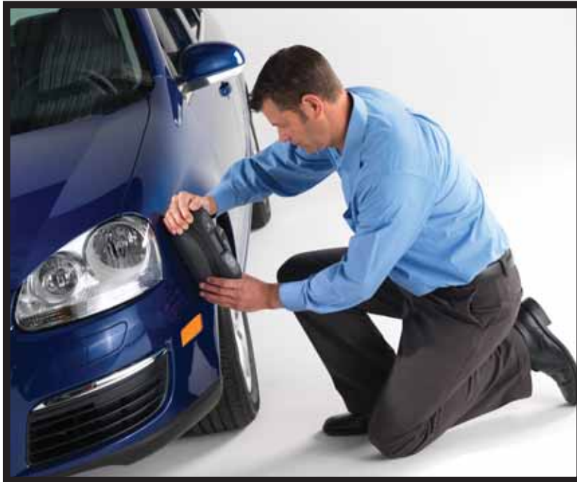
Mahr-Federal hand-held surface inspector detects surface flaws.
