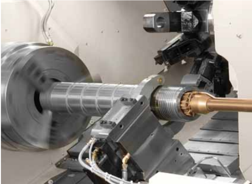
Oil pipe is being honed on a Mazak QTN 450.
