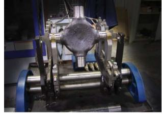
This modular bench gage is used to measure finish-machined heavy-duty truck cross trunnion parts produced on two Okuma L370 turning centers. Measurement data from the gage are processed and stored via the SPC statistical software on the machine controls. *Source: Marposs Corp.*
