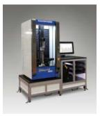
Medium volume production applications requiring an audit measuring system, or lower volume applications requiring 100% inspection are especially suited for a flexible, hybrid high precision gaging solution that integrates optical and contact technologies. *Source: Marposs Corp.*
