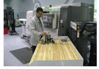
Relatively small parts produced in medium- to low-volumes are good candidates for a modular, field-retoolable "kit" type gage. Various transducers, gages, V-blocks, centers and other components can be mounted on a precision machined baseplate in virtually any configuration necessary to measure the part. *Source: Marposs Corp.*
