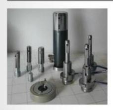
For parts that may have rough surfaces, noncontact air gages such as those shown here will be less sensitive to rough finishes and roundness due to their averaging effect; conversely, the measurement range of pneumatic gages is only about half of that available in a typical mechanical gage. Source: Marposs
