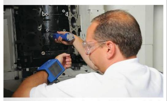
Wireless technology assists in operator convenience for taking measurements to verify parts between metal removal operations. By pushing a button, real time measurement values are displayed on the receiving electronic unit, with the possibility to store the measurement data. Source: Marposs
