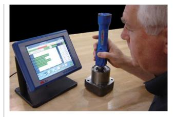
Linking a manual plug, snap or width gauge to a powerful computer with Bluetooth technology may seem like overkill, but the benefits are very real. Systems like this make it possible to migrate inspection processes upstream from the QC Lab to the machine tool, bringing manufacturing one step closer to the goal of producing a good part the first time and every time.
