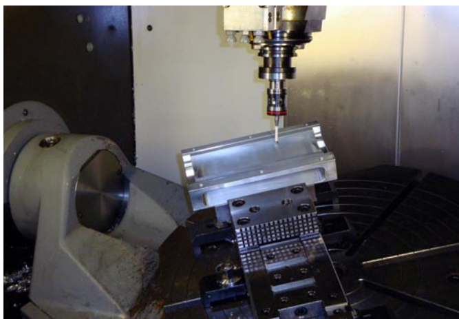
On-machine checking of mold by Marposs optical spindle probe OP32 and 3DSI
