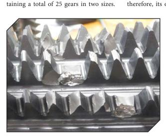
The larger gears are hobbed in 40 seconds while the smaller are produced in 4.3 seconds. Advances in tooling and machine technology have quadrupled the productivity of these operations in the last 10 years.
