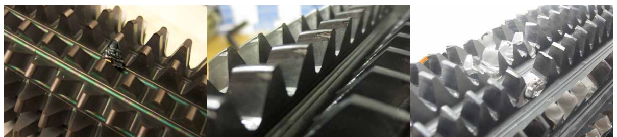
Figure 1: The Artis Tool Monitoring System couples multiple sensor inputs with software specifically designed to detect the exact kinds of anomalies produced by worn and/or damaged tools in wet and dry cylindrical gear hobbing applications
