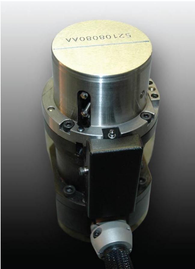
Fig. 2: A reference ball and two face contacts are located in the flange at the bottom of the nosepiece, and two reference balls are located on its circumference. The arrangement allows the part to float freely while rotating. The face contacts also allow face runout or squareness to the bore axis to be measured.
