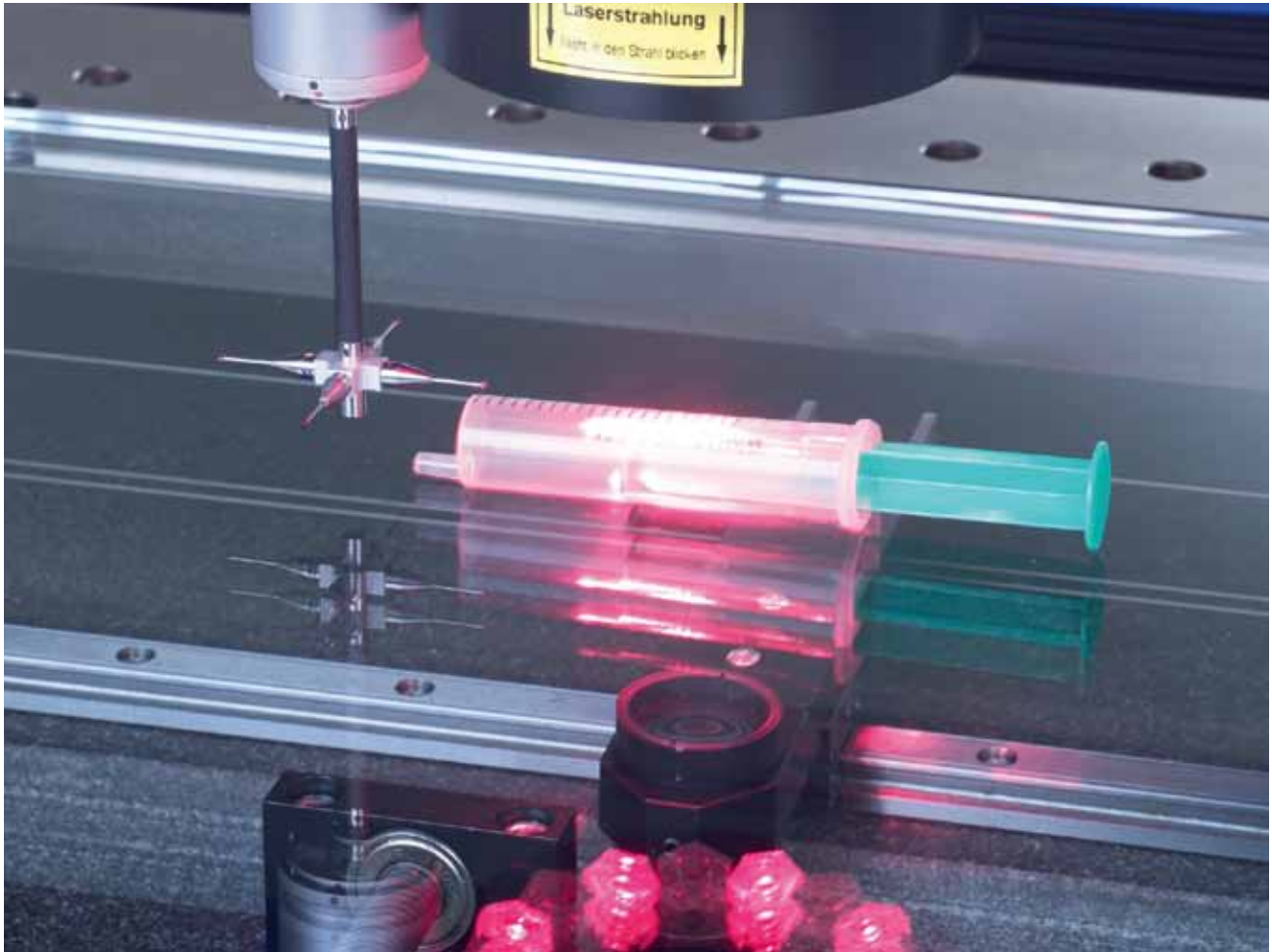
Carl Zeiss IMT's O-Inspect multisensor system with a typical medical device.
