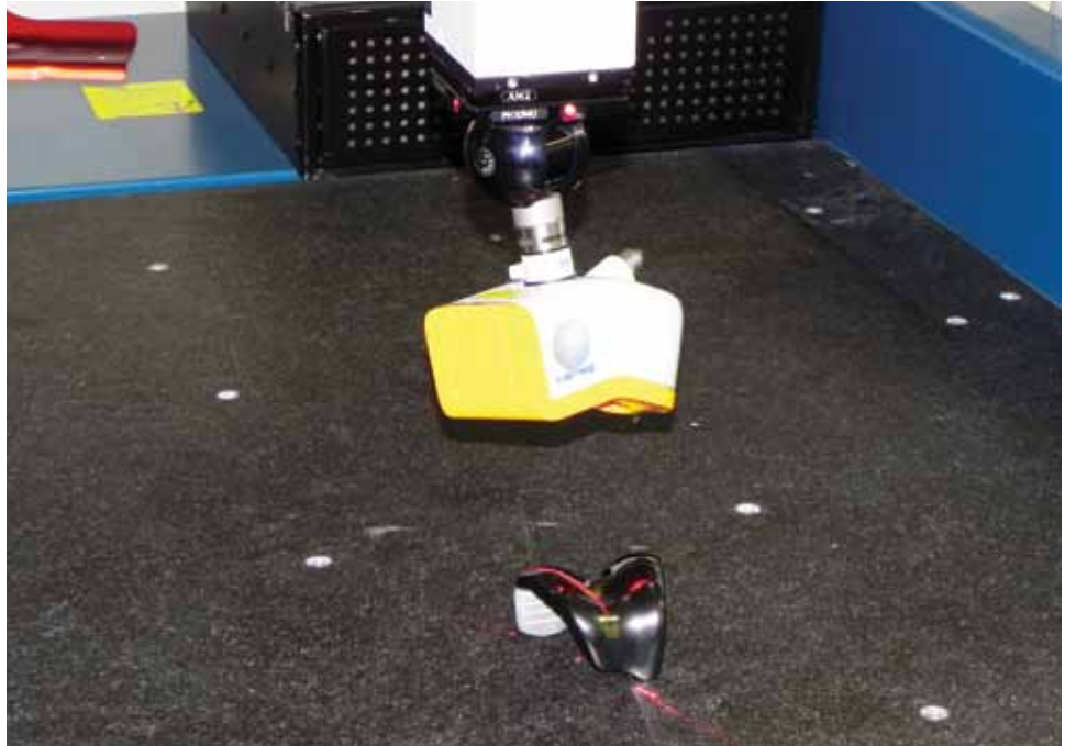
Nikon Metrology's LC60Dx collects up to 75,000 points/sec to a measuring uncertainty of 9 \mu (0.0004") at 1 sigma with measured results often as low as 7 \mu (0.0003") at 1 sigma.
