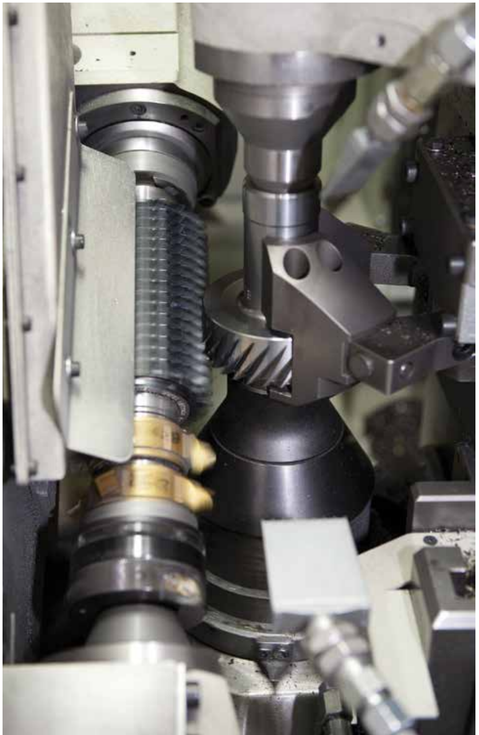
Artis couples multiple sensor inputs with software specifically designed to detect the kinds of anomalies produced by worn and/or damaged tools in wet and dry cylindrical gear hobbing applications (photo courtesy of Liebherr-Verzahntechnik).
