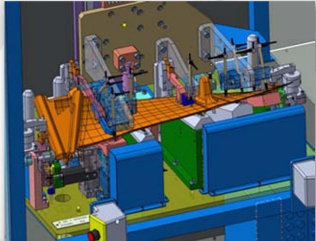
Gauging station for engine cover dimensional measurement
